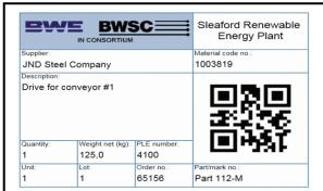
Dimensions of the label must be no less than 80 x 120 mm
